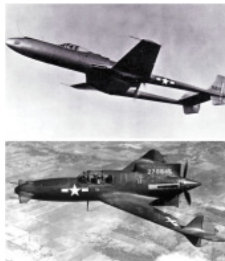
▲ The U.S. Army Air Corps' R-40C solicitation for advanced pursuit aircraft led to two other very unusual designs in addition to the Northrop XP-56 Black Bullet . At the top is the Vultee XP-54 Swoose Goose ; at the bottom is the Curtiss XP-55 Ascender .
