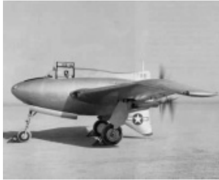
▲ Northrop test pilot John Myers runs up the first XP-56's complicated pusher engine/counter-rotating prop powerplant. Note the unpainted magnesium finish—the airplane was hardly a "Black Bullet" at rollout.
